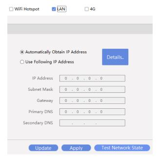
After setting, you can produce and publish programs, and manage the device via this communication method.
