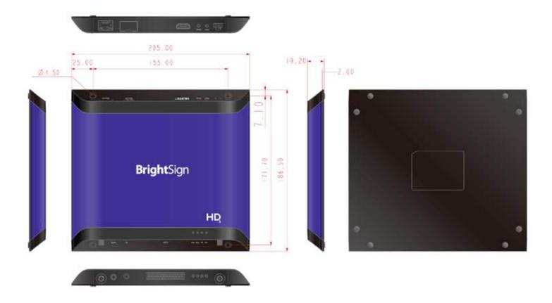
The HD225 and HD1025 can be mounted on a wall using the sealed mounting holes on the front and back. It is recommended that you mount the device using four screws (one for each hole). The screws should have a major diameter between 3.5mm and 4.2mm.
