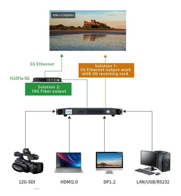
Note: When H10Fix-5G selects the output types of the four network ports, only the first two can be used.
